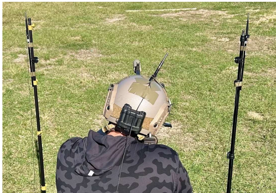
Example of Microphone and Sensor Placement while recording data for RD GPS on M240B
