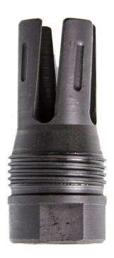
The RD KFM taper lock flash hider is our in-house designed suppressor mount. Originally designed around an agency requirement to reduce visible flash signature by 90% over a standard A2 Birdcage, with the flash hiding geometries not exceeding the form factor of the A2 Birdcage, while also acting as a suppressor host. The KFM is the smallest combination flash hider and suppressor mount we could design while meeting all of the required performance specifications.
