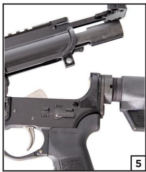
6. Remove the charging handle by pulling it backwards to keyway and then down and out of the upper receiver.
