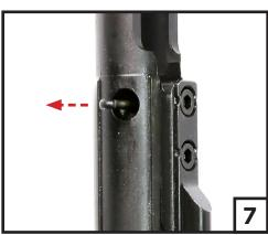
8. Tilt the bolt face up and remove the firing pin.
